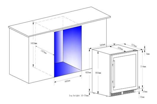
For all types of built-in product, make sure, if your appliance is placed between two pieces of furniture or in a corner against a wall, that the door opens sufficiently so that the shelves can be taken out without any problem. In fact, on some models, the doors must be opened more than 90° to pull out the shelves when removing a bottle.
